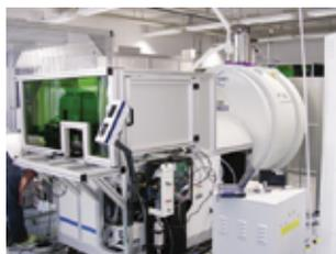
FT-ICR mass spectrometer and the tunable laser
